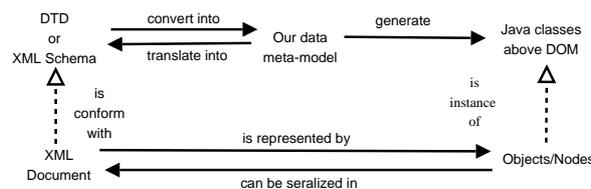
Figure 9: Bridge between data meta-models and models
