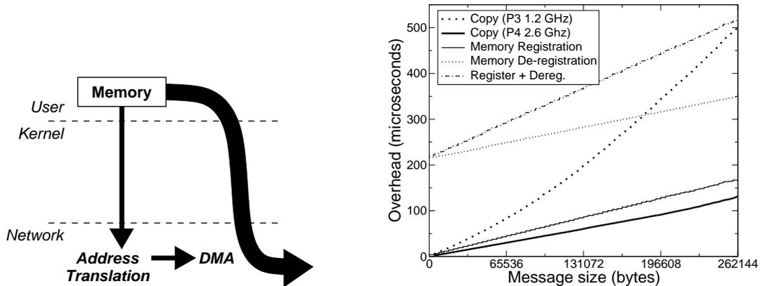
(a) DMA transfer between the application and the network after memory registration.
