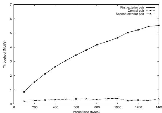
Figure 3: Achieved throughput for the three pairs configuration
