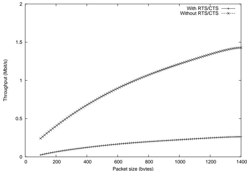
Figure 6: Throughput on a six-hops chain
