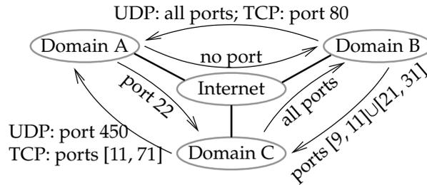
Figure 3: Grid C: firewalls limiting network traffic selectively.
