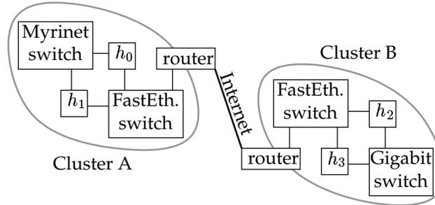
Figure 2: Grid B: overlapping of various network technologies.
