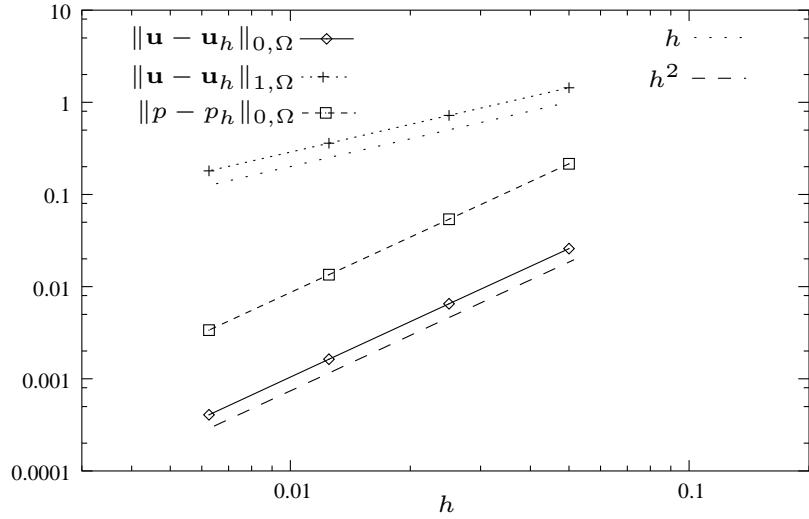
Figure 1:  $P^1$  convergence history:  $\sigma = 1$ ,  $\nu = 1$ ,  $\mathbf{a} = (1, 1)$ ,  $\lambda = 0$
