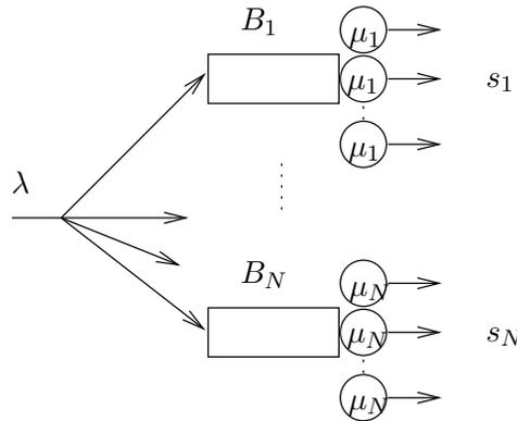
Figure 1: Queuing model of a Computational Grid with Resource Broker. The Grid is composed of  $N$  clusters (or queue), the  $i^{th}$  queue being composed of  $s_i$  CPUs (or servers) of speed (or rate)  $\mu_i$ . The system input of rate  $\lambda$  is routed amongst the  $N$  queues.
