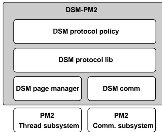
Figure 1: Overview of the DSM-PM2 software architecture.
