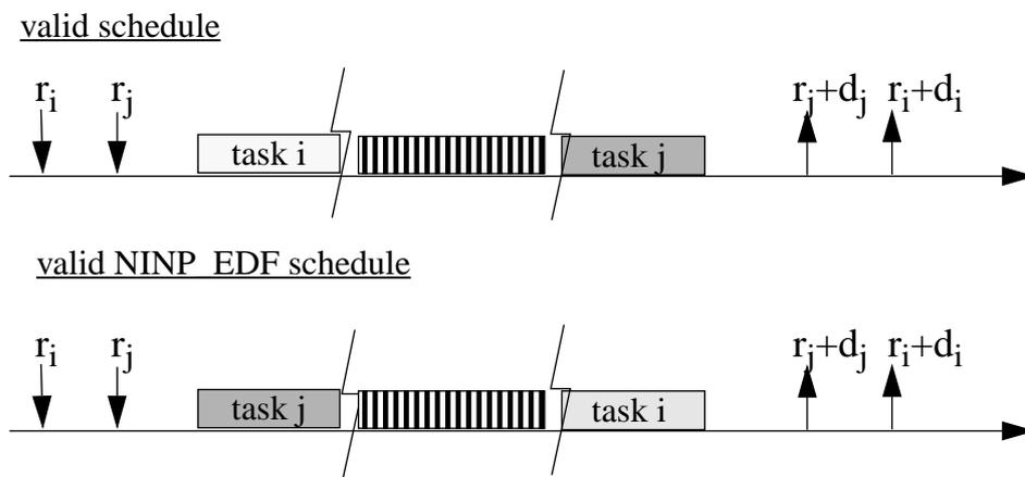
Figure 3.2: Reranking of task  $i$  and  $j$ .
