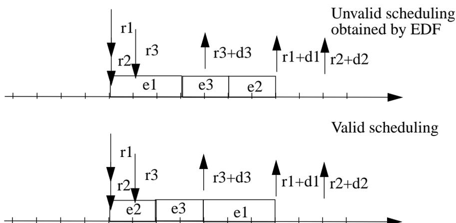
Figure 3.1: EDF is not optimal in non preemptive scheduling
