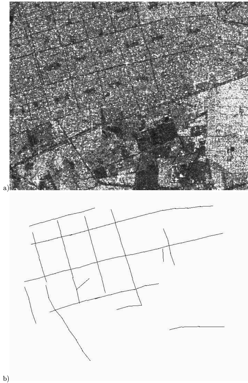
Figure 14: Extracting roads on a ERS radar image : a) original image b) the final result INRIA
