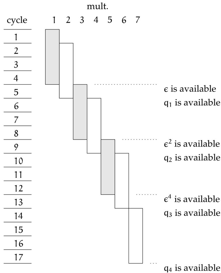
Figure 1: Schedule of the original G-iteration. It requires 17 cycles to get the final result. It allows interlacing of two independent divisions: it suffices to start multiplication **mult. 1** of the second division at cycle 3, **mult. 2** at cycle 4, **mult. 3** at cycle 7, **mult. 4** at cycle 8, **mult. 5** at cycle 11, **mult. 6** at cycle 12, and **mult. 7** at cycle 16. Two interlaced divisions require 19 cycles.
