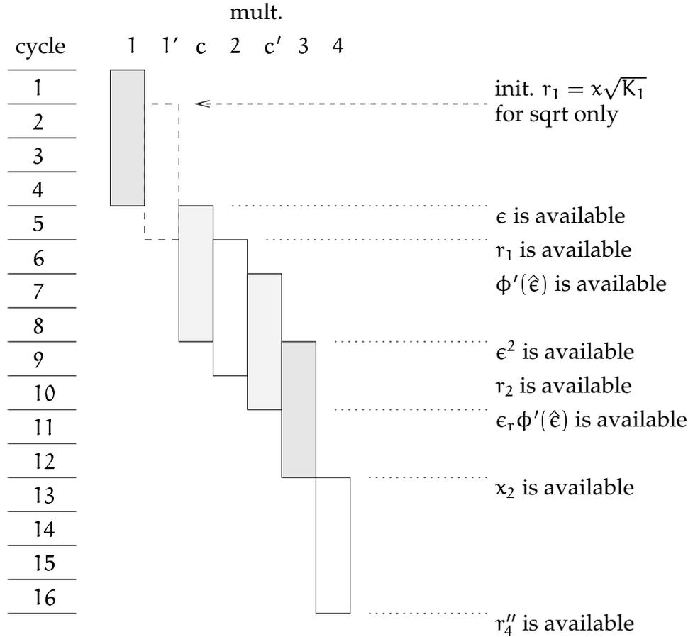
Figure 4: Implementation of  $\sqrt{x}$  and  $1/\sqrt{x}$  on a 4-cycle pipelined multiplier. Mult. 1' is performed only for  $\sqrt{x}$ ; c and c' correspond to the computations of  $\epsilon^2$  and  $\epsilon_r \phi'(\hat{\epsilon})$ .
