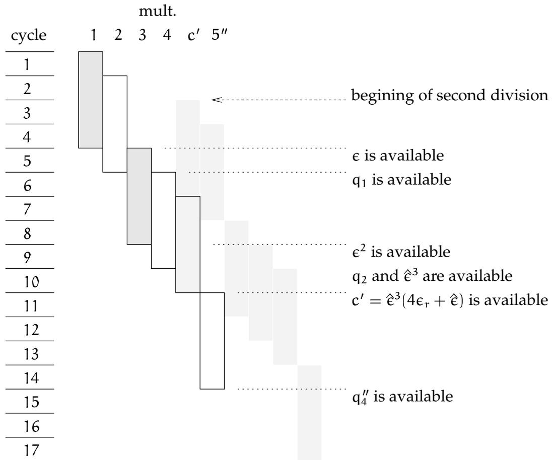
Figure 3: Variant B. Mult.  $c'$  is the computation of  $\hat{e}^3(4e_r + \hat{e})$ . Mult.  $5''$  is the final multiplication. It has one more cycle than Variant A, but the accuracy is much better. Two interlaced divisions need 17 cycles.
