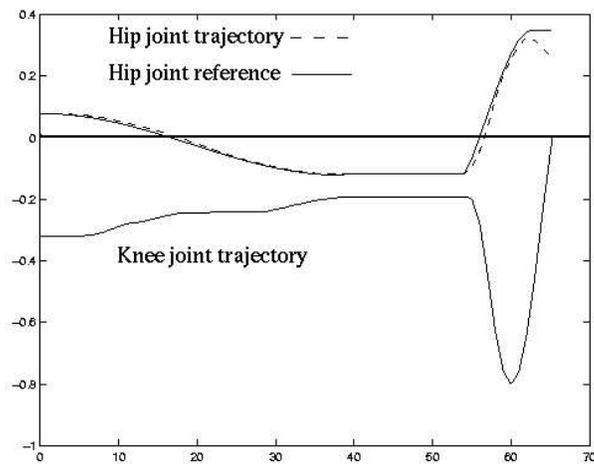
Figure 6: Trajectories of joint variables during the swing phase
