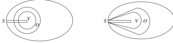
Figure 2: Neighbourhoods of the crack tip
