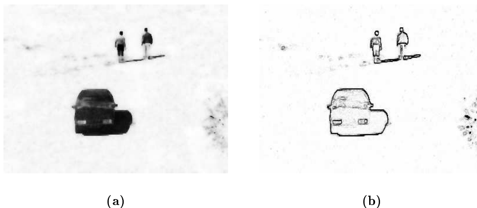
Figure 4: Results concerning moving objects detection (a) Function C(x, y, t) at a given time and (b) its dual variable associated d_C .
