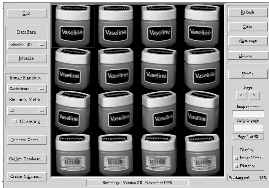
Figure 10: Retrieval of the top left image. Note that among the best matches are rear views of the vaseline bottle
