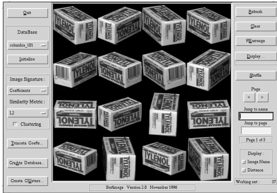
Figure 12: Retrieval of the TYLENOL pack on the top left by using the nearest cluster. All retrieved images are TYLENOL packs
