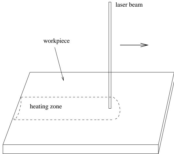
Figure 1: Sketch of a laser hardening process
