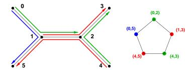
Figure 1: A routing for five requests in a tree and its associated conflict graph.
