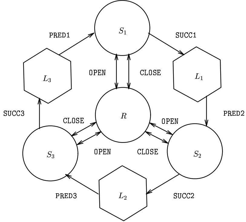
Figure 3: Ring with three stations *S<sub>i</sub>* and three links *L<sub>i</sub>*
