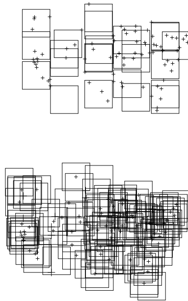
Figure 3: Finding a covering of 120 cities of the U.S.A. Our algorithm reports a set of 25 unit squares covering the 120 cities. Any solution requires at least 11 squares. (Considering the corresponding piercing problem, one may find 11 disjoint squares.)
