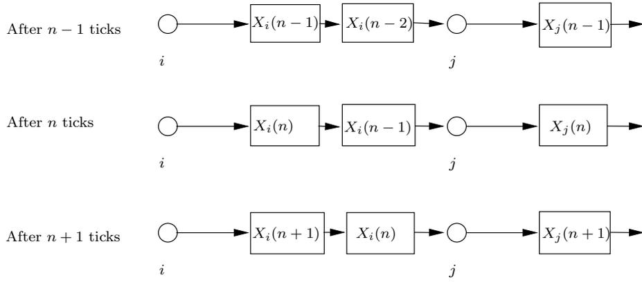
Figure 14: Digital circuit computing  $X_j(n) = F_j(X_i(n-2), \dots)$ .
