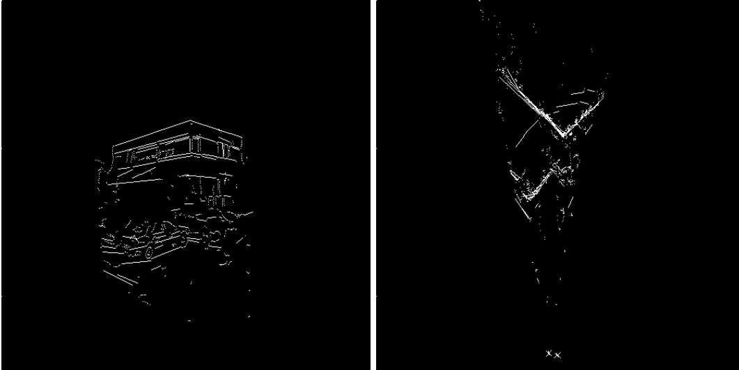
Figure 13: If we fit lines to the image edge data and then reconstruct using method 3 we can recover a more accurate and reliable understanding of the three-dimensional geometry. Furthermore, we can begin to reason about the more general world structure such as searching for connectivity and coplanarity constraints. The two camera positions are marked in the lower part of the right hand image, and points that are not suitably represented by lines are reconstructed as isolated points.
