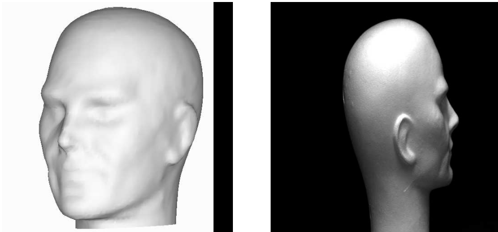
Figure 11: Left: The 3D model of the mannequin head. It was extracted from a 3D CT-scan image. Thanks are due to Cannes Hospital. Right: A video picture of the mannequin head. Our goal is to find the point-to-point correspondence between the left and the right objects.
