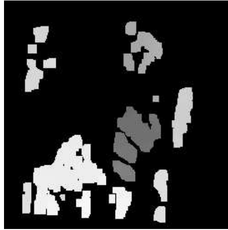
Figure 6: The disparity map obtained from the rectified images of figure (5).
