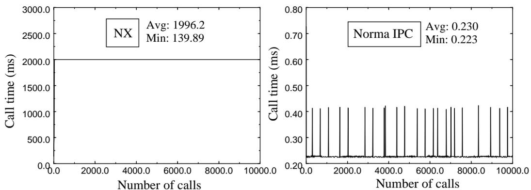
**Fig. 10: Performance of inter-process (intra-node) communications using NX and Norma IPC**
