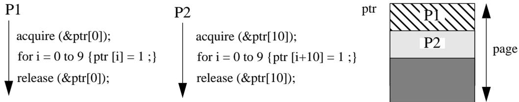
Fig. 5: Use of the page locking mechanism
