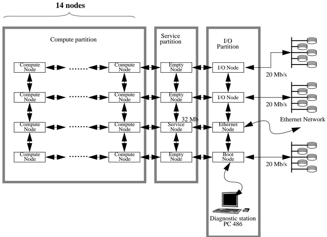
**Fig. 1: The Intel Paragon hardware configuration at IRISA**
