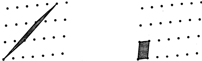
Fig. 1. A lattice and two of its bases represented by the parallelogram they span. The first basis is skew, the second one is reduced.
