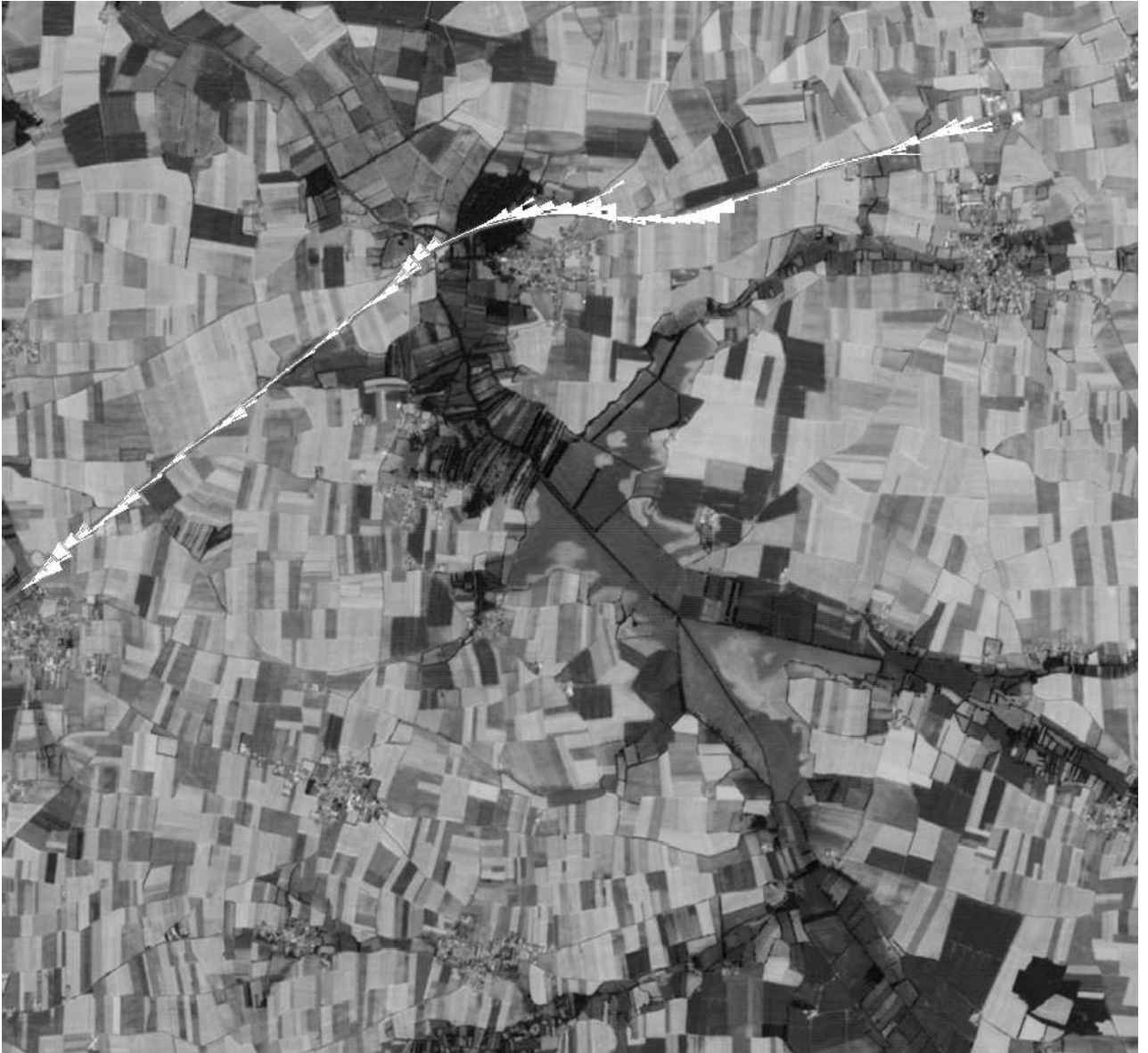
Figure 5: Tracking results on a SPOT image from La Rochelle, France. The arcs selected by the algorithm are shown in white.
