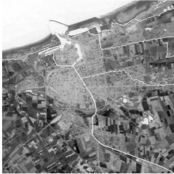
Figure 13: Segmentation of the roads and channels in r_1 with cliques of order three and a static model - first test
