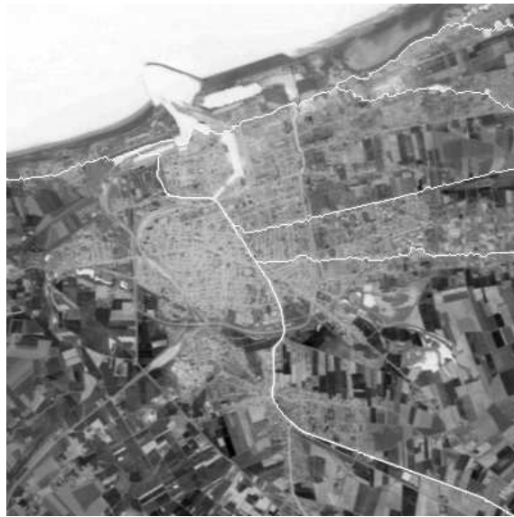
Figure 14: Segmentation of the roads and channels in r1 with cliques of order three and a static model - second test
