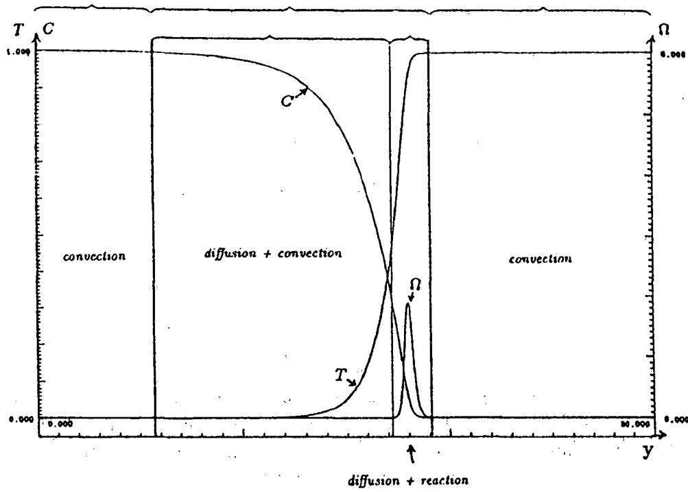
Figure 2.1: Structure of premixed flame
