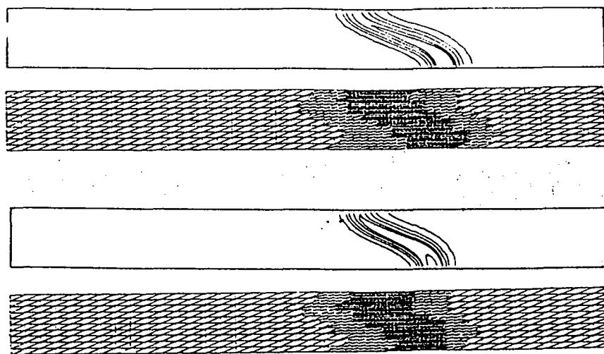
Figure 5.12: FEM error for a semi-infinite duct with coefficients coming directly from the equation system
