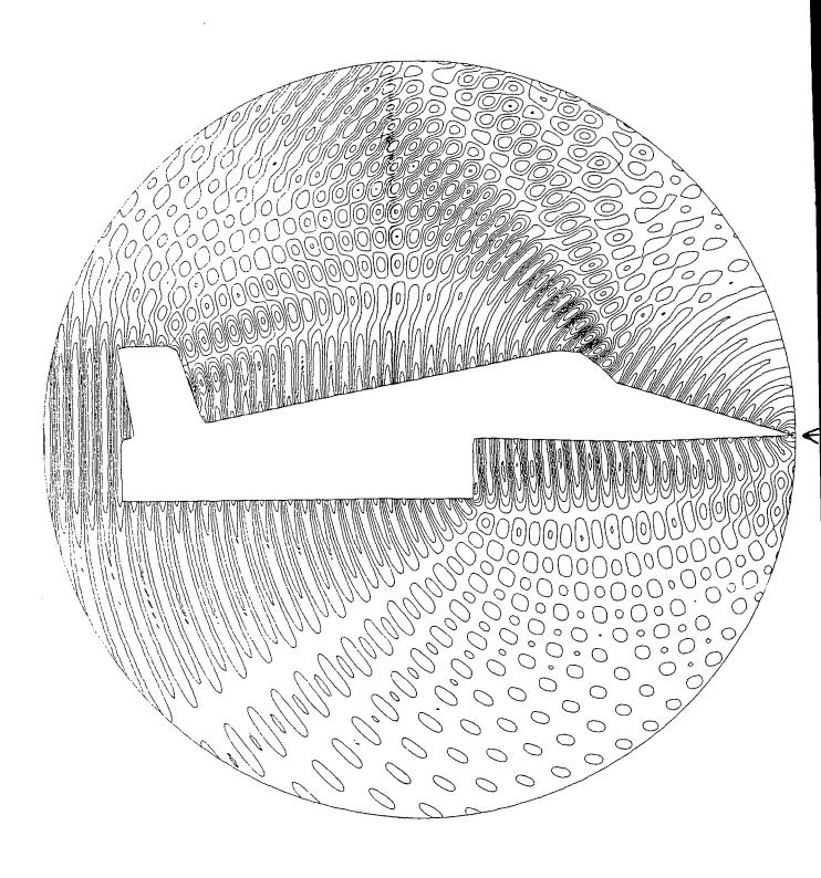
Figure 8. Solution for the airplane-like obstacle  $\omega=8,~\alpha=0^{\circ},~n_r=130,~n_\theta=750,~N_0=83250$  10 isolines of the real part
