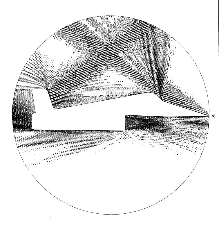
Figure 10. Solution for the airplane-like obstacle  $\omega=30,~\alpha=0^{\circ},~n_r=518,~n_{\theta}=3200,~N_0=1414400$  10 isolines of the real part
