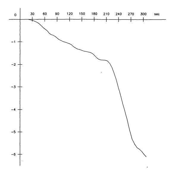
Figure 2.  $\log_{10}\frac{\|\xi\|_2}{\|f\|_2}$  versus CPU time for the  $\Pi$ -shaped open resonator  $n_r=47,\ n_\theta=280,\ N_0=13161,\ \alpha=30^\circ$  The computer - Apollo DN5500
