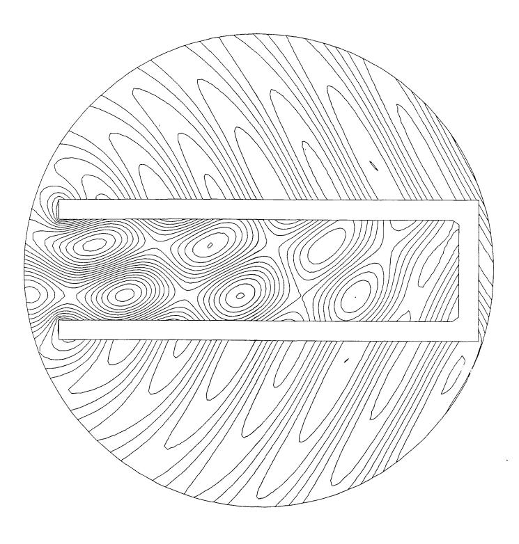
Figure 3. Solution for the  $\Pi$ -shaped open resonator  $n_r=47,\ n_\theta=280,\ N_0=13161,\ \alpha=30^\circ$  20 isolines of the real part  $\min=-2.817,\ \max=2.721$
