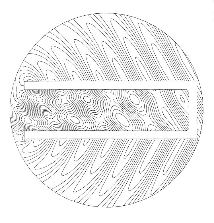
Figure 4. Solution for the  $\Pi$ -shaped open resonator  $n_r = 47$ ,  $n_\theta = 280$ ,  $N_0 = 13161$ ,  $\alpha = 30^\circ$  20 isolines of the imaginary part  $\min = -2.382$ ,  $\max = 2.218$
