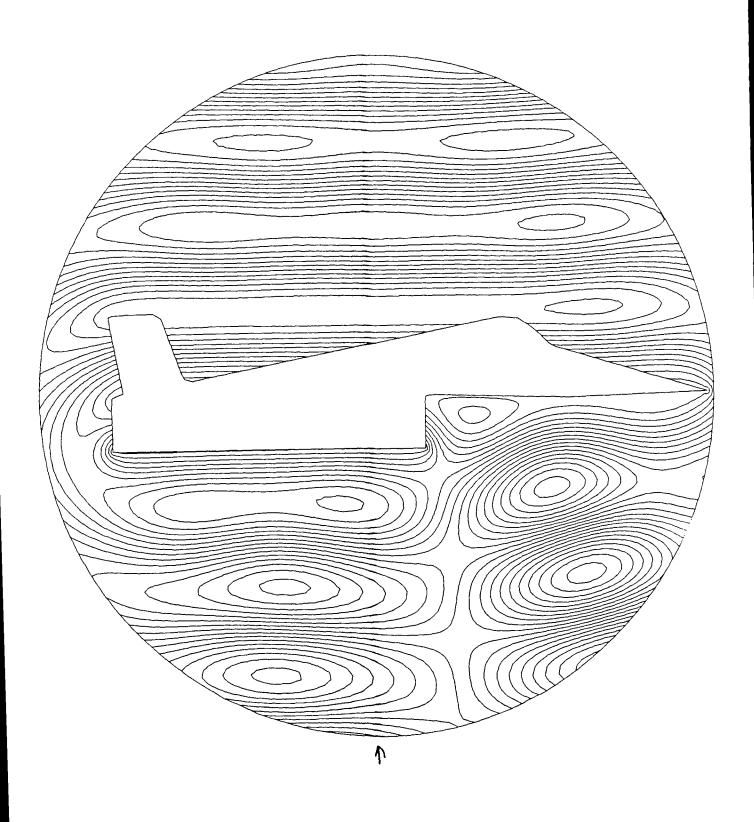
Figure 7. Solution for the airplane-like obstacle  $\omega=1.2,~\alpha=90^{\circ},~n_{r}=53,~n_{\theta}=320,~N_{0}=14400$  20 isolines of the real part
