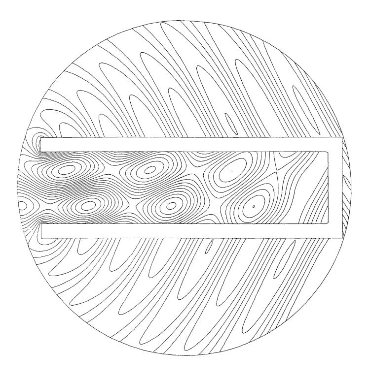
Figure 5. Solution for the  $\Pi$ -shaped open resonator  $n_r = 93$ ,  $n_\theta = 560$ ,  $N_0 = 52081$ ,  $\alpha = 30^\circ$  20 isolines of the real part  $\min = -2.990$ ,  $\max = 2.924$
