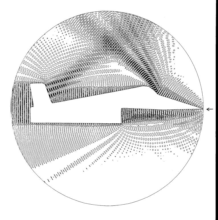
Figure 9. Solution for the airplane-like obstacle  $\omega=15,~\alpha=0^{\circ},~n_{r}=259,~n_{\theta}=1500,~N_{0}=330000$  10 isolines of the real part
