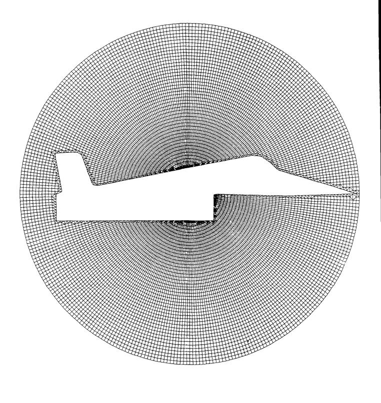
Figure 6. The locally fitted mesh for the airplane-like obstacle
