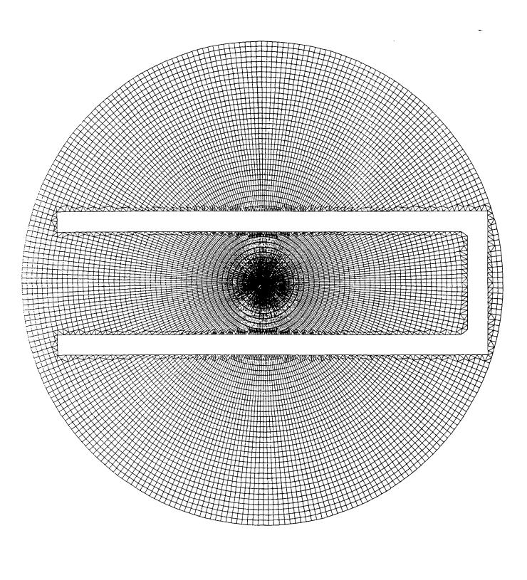
Figure 1. The locally fitted mesh for the  $\Pi$ -shaped open resonator
