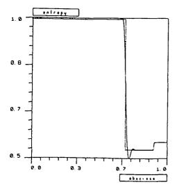
figure 2 : sod shock tube . 200 points . second order scheme with centered , non\_limited slopes .
