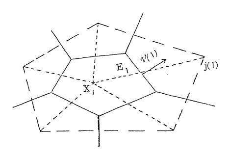
figure 1:an example of unstructured mesh.
