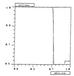
figure 3: sod shock tube. 200 points. second order scheme with the only limitation on the entropy (6).
