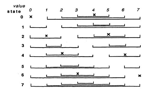
In the first state, the processor ctrl triggers (by sending a signal) the communications between processors 1 and 7, 2 and 6, 3 and 5; processors 0 and 4 remain inactive. When a processor has finished its computation, it sends a signal to the controller. So when the controller has received n signals, the current step is over and a new signal is spread over the network (if the termination state is not yet achieved).
