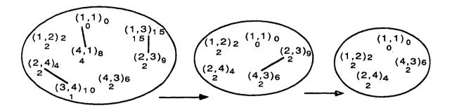
The final state of M represents the tree of the shortest paths from vertex 1 to vertices 2,3 and 4.
