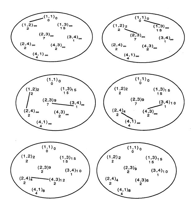
The final multiset M1 may contain tuples  $(i,a)_{li}$ ,  $(j,a)_{lj}$  where  $i \neq j$ . In order to define the ci cj shortest path, it is necessary to keep only the tuple  $(k,a)_{lk}$  with  $lk = Min \ lj \ s. \ t. \ (j,a)_{lj} \in M1$ .
