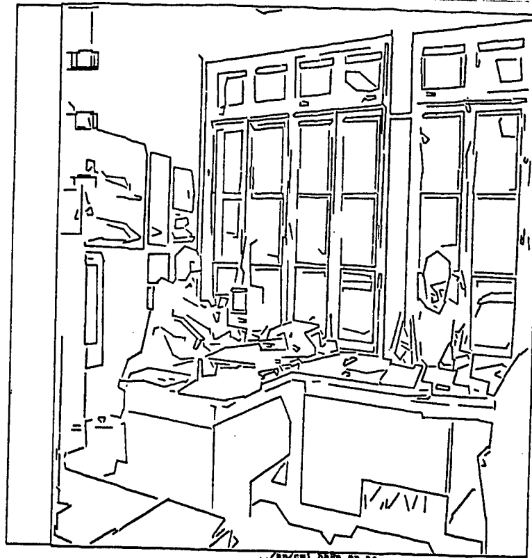
Figure 13: Polygonal approximation of the edge points of a stereo pair of the same office room observed in position 2
