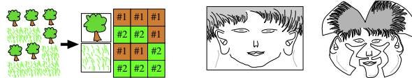
Figure 2: left : A tiling allows to save memory by instancing a small set of patterns. right : A texture atlas releases distortions by allowing mapping discontinuities.
