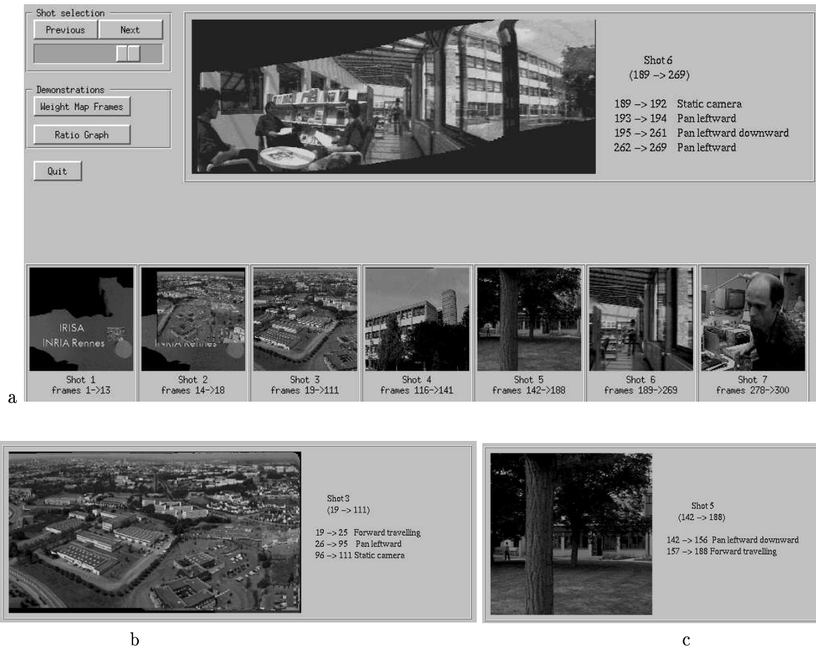
Figure 7: IRISA sequence: visualization of the video summary (a). A key-frame per detected shot is displayed (bottom row), and, for a user-selected shot, more information about its contents is supplied (mosaic image and sequence of camera motion types). Examples shown correspond to (a) shot 6, (b) shot 3 and (c) shot 5.
