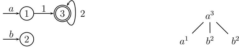
Fig. 6. An stepwise tree automaton over \{a, b\} recognizing \{a(w) \mid w \in L(ab^*)\} and one of its successful runs. Initial states for a are pointed to by arrows labeled by a . The state 3 of the root is obtained by running the automaton with initial states for a on the string 122.
