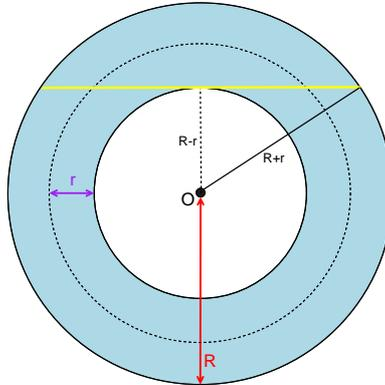
Figure 5: Viewing a torus from top. We show how the longest ray's length (in yellow) can be easily computed from the tokamak's parametric equation.  $r$  is the minor radius and  $R$  the major radius of the torus.
