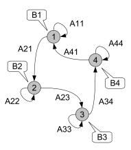
Figure 3. A HMM as a probabilistic automaton. Each state is associated with an emitted signal.
