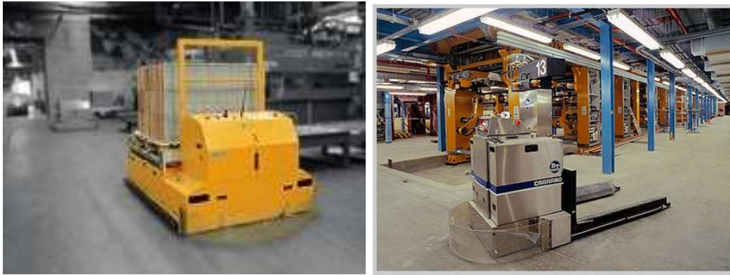
Figure 5: Automated forklifts: Frog Palette Mover (left) and BT Industries Autopilot (right).
