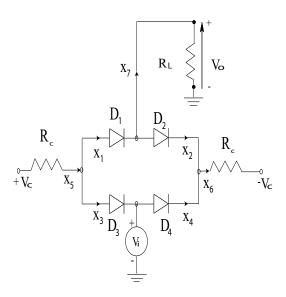
Figure 18: four-diode-bridge sampling gate
