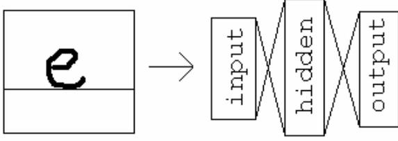
**Figure 2.** The baseline recognition architecture is a simple feed-forward neural network. The ink is featurized and normalized into 64 feature vector which is used as input to the neural network. The output layer of the neural network has 99 nodes, one for each character supported. The activation of each output node corresponds to the probability the ink is the character corresponding to that output node.
