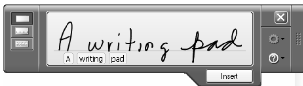
Figure 1. A typical input pad layout is shown. This UI is used on a keyboard-less device to provide a natural text input mechanism. The user writes in the input area with a pen and a handwriting recognizer converts the ink into text.
