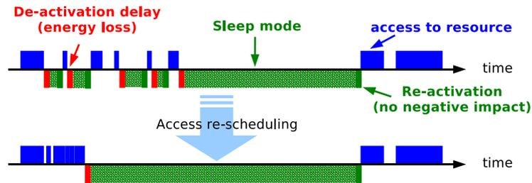
A specific case of access re-scheduling can be performed at loop level. Loop fission consists in splitting 1 loop into several loops, when the instructions in the original loop do not depend on each other. The various loop can thus process different pieces of data (arrays...), which offers a better locality and increases sleep mode opportunities [7, ch10].
