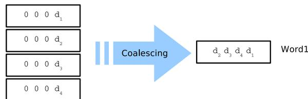
Lifetime analysis is a dual approach allowing “temporal coalescing”. It consists in putting in the same slot pieces of data that do not coexist at the same time, even though each piece completely fills the slot.
