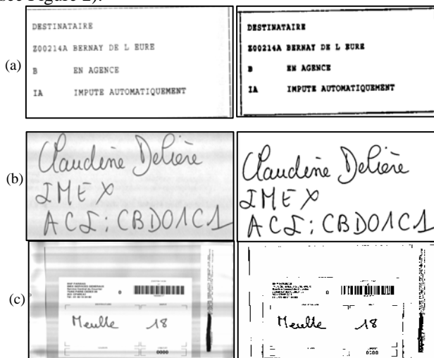
Figure 2: Thresholding by the Sauvola's local method, (a) CHC Image, window 7x7, (b) (CIM) Image, window 9x9, (c) 'Insert' Image, window 15x15.
