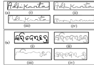
Figure 11. Examples of some images for Fractal feature computation (a) English (b) Oriya (i) Original image (ii) Full contour (iii) Upper contour (iv) Lower contour.
