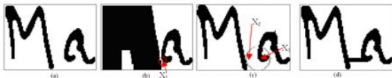
Figure 8. Joining of isolated characters in a word image is shown (a) A word containing two isolated characters. (b) The grown version of the left component and touching point ( X_1 ) in the right component is shown. (c) From X_1 the point ( X_2 ) on the first component is shown for joining. (d) Joined version of the word.
