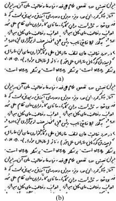
Figure 2. (a) Space between words and lines is normalized and the padding is done for each line of text, (b) the final preprocessed image
