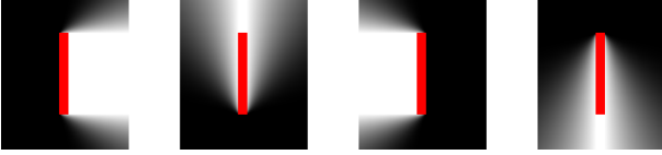
Figure 3. Fuzzy landscapes for the directional relationships right_of , above , on_the_left and below relatively to the object R presented in figure 1 (high grey values correspond to high membership values).
