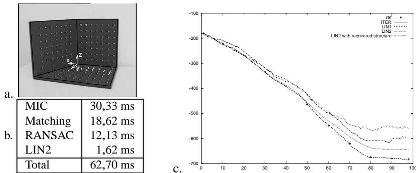
Figure 1: (a) One snapshot of the target sequence (b) Computation time (c) Temporal evolution of  $t_x$  with three planes, for ITER, LIN1, LIN2 and LIN2 with the recovered structure. The crosses represent the actual values of  $t_x$
