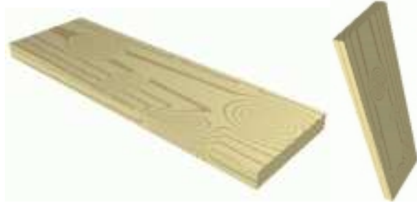
Fig. 10. Simulation of a sawed board using the implicit method.
