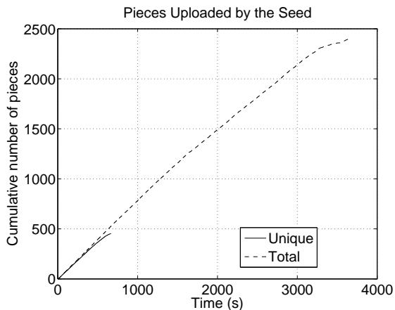
Figure 8: Number of pieces uploaded by the seed, for a single representative run. The Unique line represents the pieces that had not been previously uploaded, while the Total line represents the total number of pieces uploaded so far. The seed is limited to 200 kB/s. We observe a 16% duplicate piece overhead.
