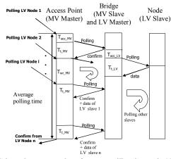
Fig. 4. Schematic representation of average polling time at the Network Layer level in REMPLI PLC network
