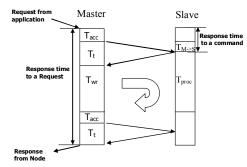
Fig. 2. Schematic representation of application-to-application delay at the Network Layer level in an autonomous PLC network
