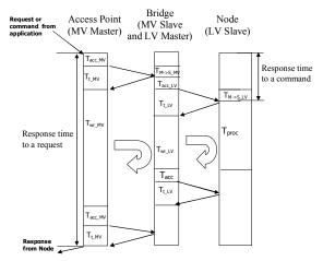
Fig. 3. Schematic representation of application-to-application delay at the Network Layer level in REMPLI PLC network
