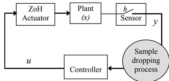
**Figure 1. Closed loop control system with sample dropping process**
