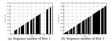
Figure 8: Evolution of sequence number of packets on the output port (1000 Mbps + 1000 Mbps (1500 bytes) on Foundry switch)
